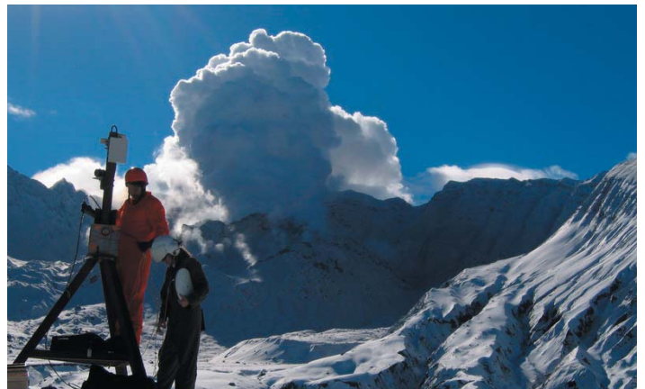
Setting up a new GPS station north of the active dome (seen steaming away in the background).
